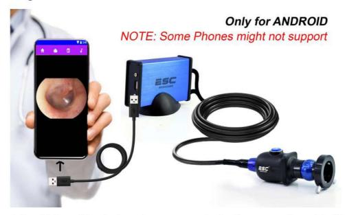
Connect the Yellow Socket and power socket of camera head to Video input & power input plug of USB adapter.
